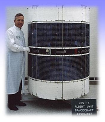
these birds in geostationary orbits approximately 22,000 miles above earth where they could each envision almost half the globe. With any pair of LES birds, communications between two points on the ground could most likely be accomplished. The threat of jamming would still exist, but finding the right two satellites and narrowing down the frequencies being used would be a significantly more difficult task for even a technologically sophisticated enemy.
