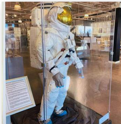
Space suit and life-support backpack used by astronauts during moon landings
