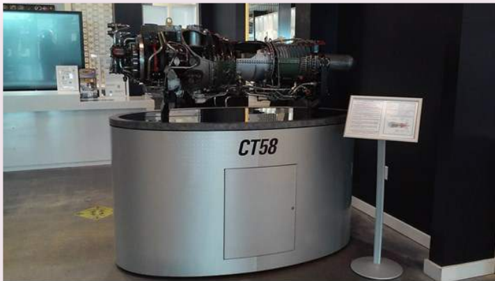
The General Electric T58 is an American turboshaft engine developed for helicopter use
