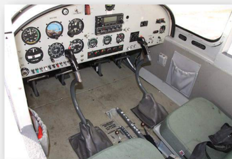
Thurston Teal cockpit with stick controls, and manual main and tail gear controls.
